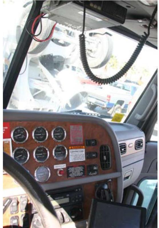
*A mobile radio fixed to the roof of the cab provides voice communications, plus its modem connects a data terminal and computer display mounted on an extension from the console. In operation, the terminal has a large status display with GPS reporting and the screen allows drivers to see their jobs being delivered to them.*
