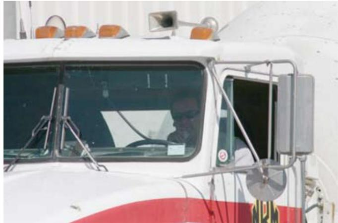
*Delivery truck drivers have the option of communication with the dispatcher by voice radio, but most communications are carried by the mobile data system. The system automatically transmits the trucks' location and the condition of the concrete it carries. In addition, a monitor in the cab displays instructions and other information of the driver.*
