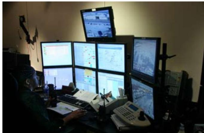
*In addition to displays with details for orders in process, trucks en route and the condition of the trucks' individual loads of ready-mixed concrete, the dispatcher can watch truck movements in the batch plants using cameras that send video to several monitors.*
